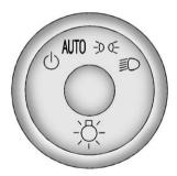
The exterior lamps control is located on the instrument panel, to the left of the steering wheel. : Turns the automatic light control on or off.
